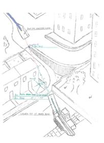
park. The solution involved a directionally drilled route of 30m, drilled at a minimum depth of 2m, housing the 500mm PE pipe, from St Anne's Road to Lantern Close.
